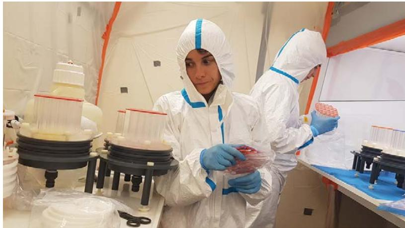
In the bubble, Marion and I take care of in-situ pumps. These pumps filter big quantities of water (up to 1000L) through filters. We deploy around 10 in-situ pumps on a cable off the ship.
