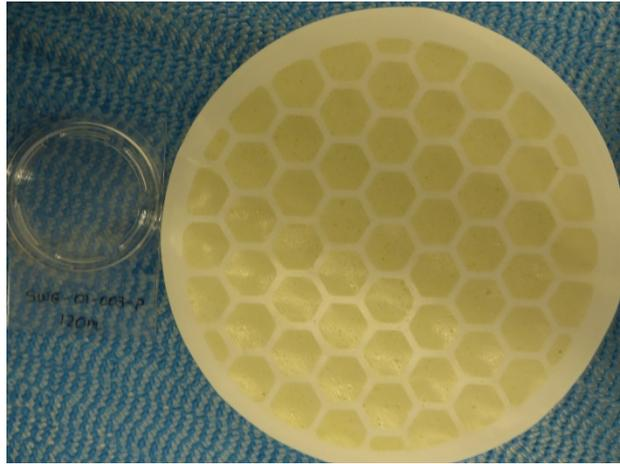
An unused filter is all white and on that one, you can see some brown marks: those are particles! There are many different particles: they can come from biology (phytoplankton, fecal matter), from sediments, from margins, from atmospheric dusts, etc.. We can see these different types of particles via the colours of the filters after filtration:
